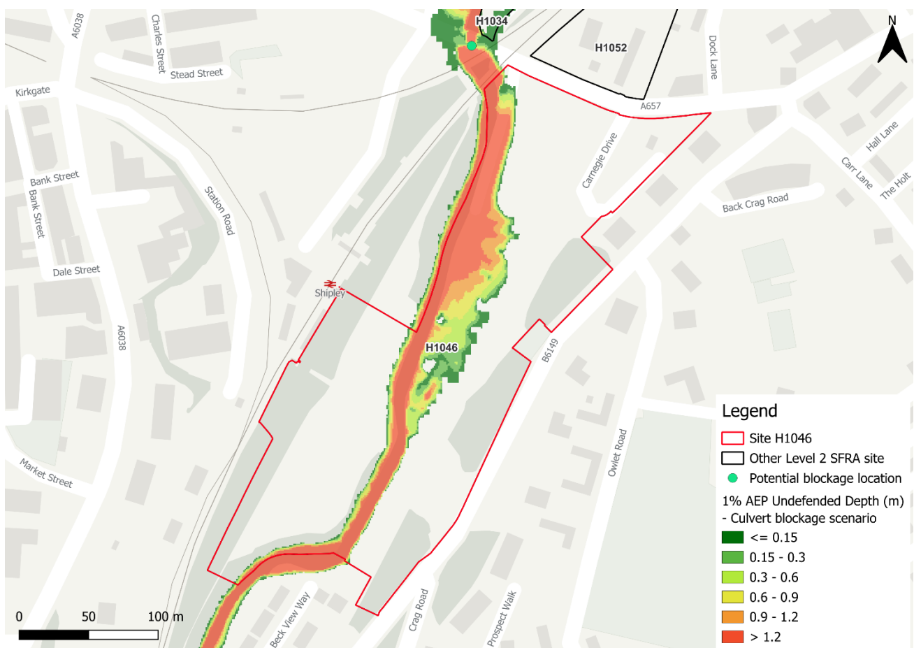
Figure 5-1: Flood depths for 1% AEP undefended flood event 50% culvert blockage scenario - structure beneath Leeds Road (A657)
